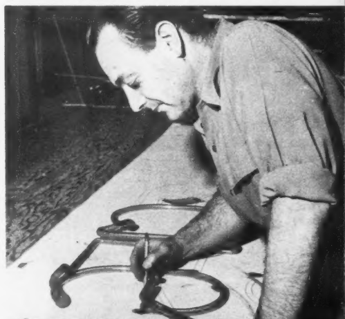
A skilled "patcher" traces a section of tubing on an asbestos pattern to finish up a missing part. Below, here's what they DID blow up on Broadway.
